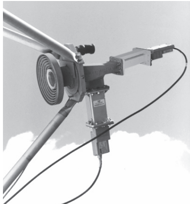
Photo of 7893D (7894D) mounted between antenna feed and LNA's (both Vertical and Horizontal Polarization.)
